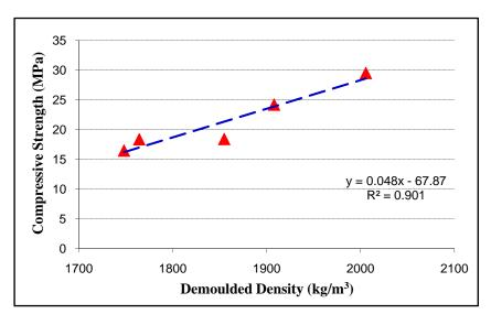
Figure 4: Correlation between Demoulded Density and Compressive Strength of Pumice Breccia Lightweight Concrete
